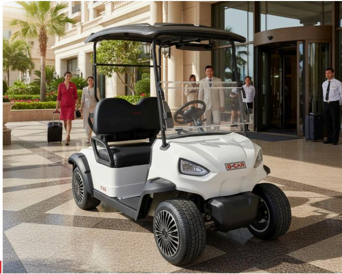
The Q-CAR PAR is a dependable entry-level two-seater electric golf car designed to enhance every round with effortless performance. Blending reliable engineering with sleek style, it features a foldable windshield, robust 12" steel wheels with hubcaps, a powerful 5kW AC electric motor, and a long-lasting 150Ah Lithium Iron Phosphate (LiFePO4) battery. The PAR model is fully customisable to meet the specific needs of any club's fleet requirements.
