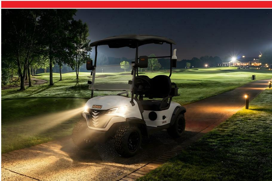
The Q-CAR BIRDIE exemplifies the pinnacle of premium two-seater golf cars, integrating sophisticated design, state-of-the-art technology, and exceptional performance. Powered by a robust 5kW AC electric motor coupled with an advanced 150Ah Lithium Iron Phosphate (LiFePO4) battery system, the BIRDIE ensures smooth and quiet operation with minimal maintenance requirements.
